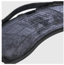
**Auger:**Very high wear during the tests (completely)
